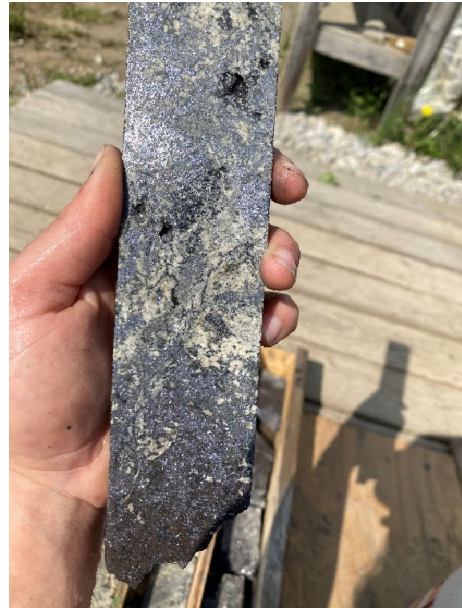
Photo 5. WPC22-07 Massive interstitial argentiferous galena with minor sphalerite in-filling a dolomite crystal mat
