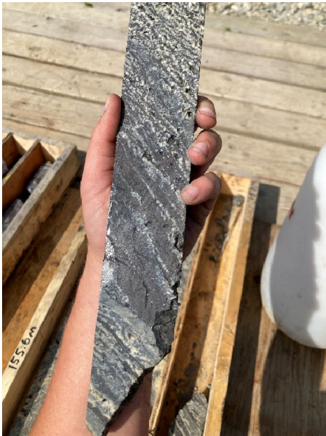
Photo 3. WPC22-07 Banded 'Zebra' Mineralization Bands of massive Fe-rich sphalerite and/or argentiferous galena between laminated dolomite crystals
