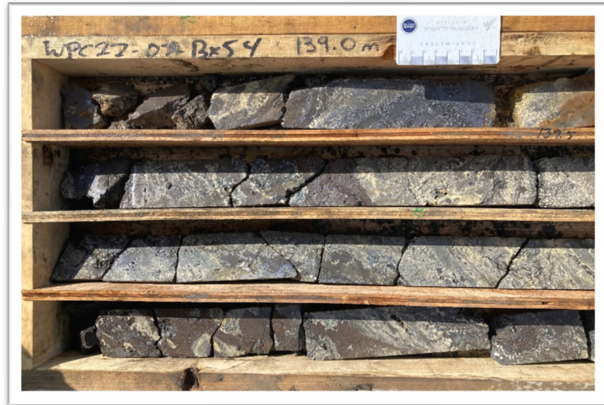
Photo 1. Portion of Upper Massive Sulfide Interval WPC22-07 138.0-143.5 meters - 4.5 meters Massive Intergrown Sphalerite, Argentiferous Galena and Recrystalline Dolomite
