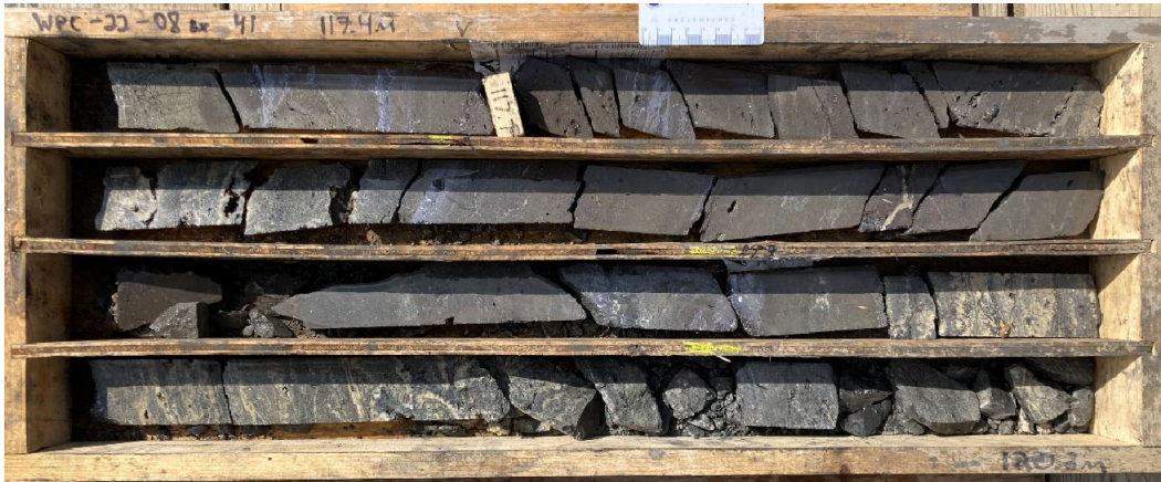
Photo 7. Portion of massive sulfide Interval WPC22-08 114.6-123.1 meters - 8.5 meters Massive Sulfide Mineralization with Fe-rich Sphalerite and Bands of Argentiferous Galena
