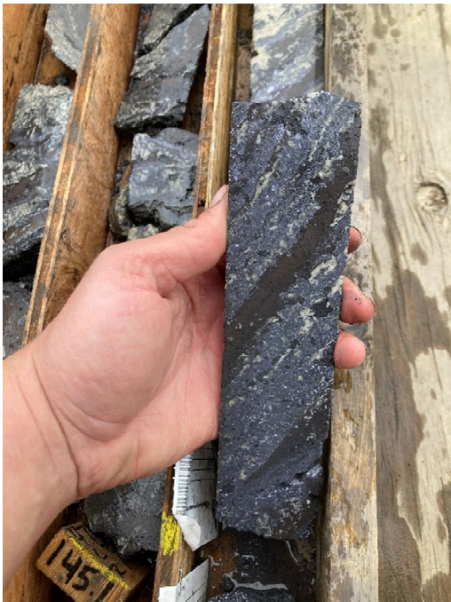
Photo 11. WPC22-11 Mat of intergrown argentiferous galena and dolomite cut by Fe-rich sphalerite bands
