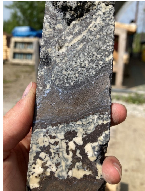
Photo 6. WPC22-07 Multiphase massive Fe-rich sphalerite mineralization with zones of late argentiferous galena infilling a mat of dolomite crystals and crosscutting earlier massive sphalerite
