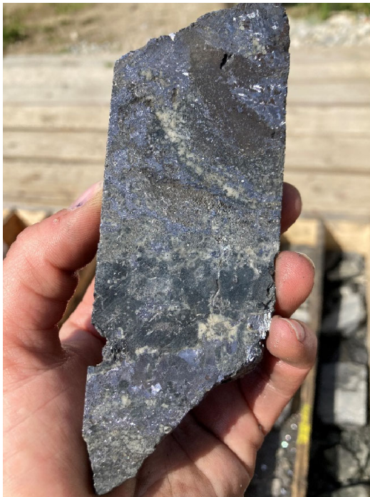
Photo 8. WPC22-08 Massive intergrown sphalerite and argentiferous galena infilling a mat of fine-grained dolomite crystals
