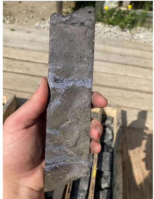
Photo 9. WPC22-08 Massive sphalerite cut by argentiferous galena veinlets
