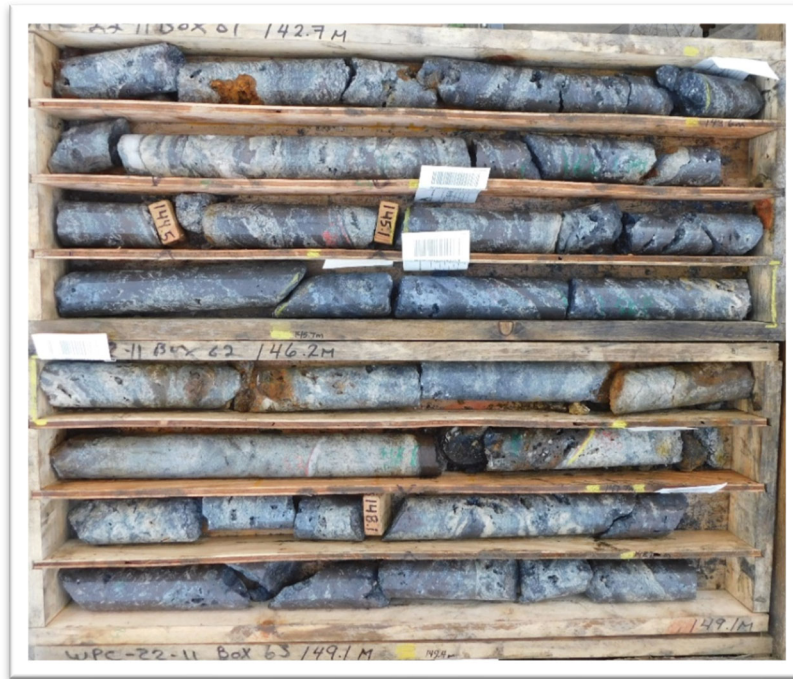
Photo 10. Portion of massive sulfide interval WPC22-11 139.1 – 150.6 – 11.5 meters
