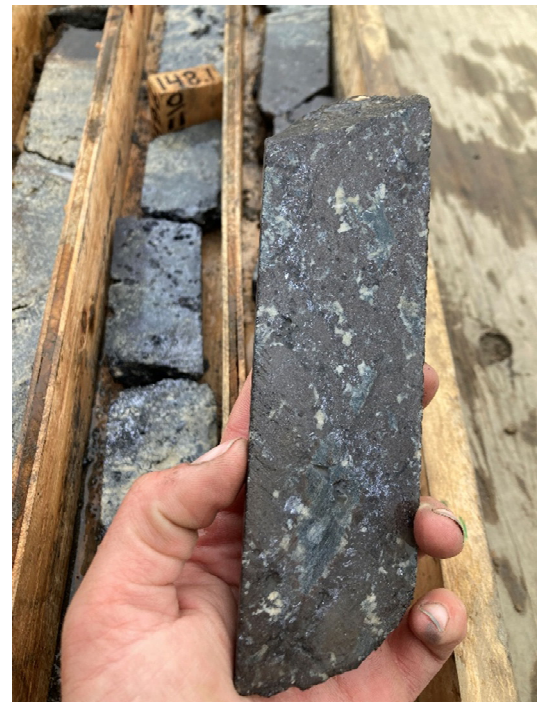
Photo 12. WPC22-11 Massive intergrown Fe-rich sphalerite with interstitial argentiferous galena
