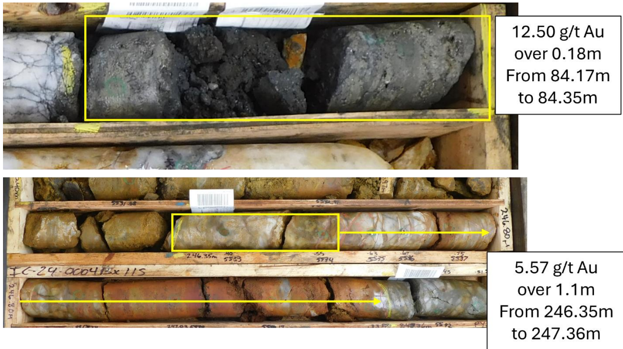
Figure 2. Massive pyrite with breccia texture for the intercept reported in Table 1.
