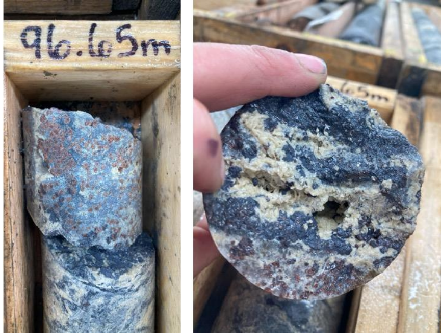
Figure 3B: Drill core from IC24-0012 shows coarse-grained red sphalerite in the recrystalline ankerite stage with galena
