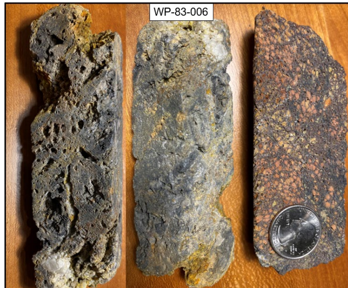
Figure 7.14: WPC Oxide Zone Drill Core: WP-83-006: 14.1m at 25.3 Oz/t Ag, 44% Pb, and 2.3% Zn
