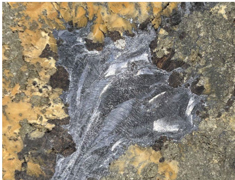
Figure 7.10: Argentiferous Galena with Pyrite, Fe-rich Sphalerite, and Dolomite: WPC22-20
